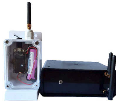
Figure 1. LoRa modules used in the experiment (in the white case – a transmitter at a frequency of 868 MHz, in the black case – a transmitter at 433 MHz and 2.4 GHz)
